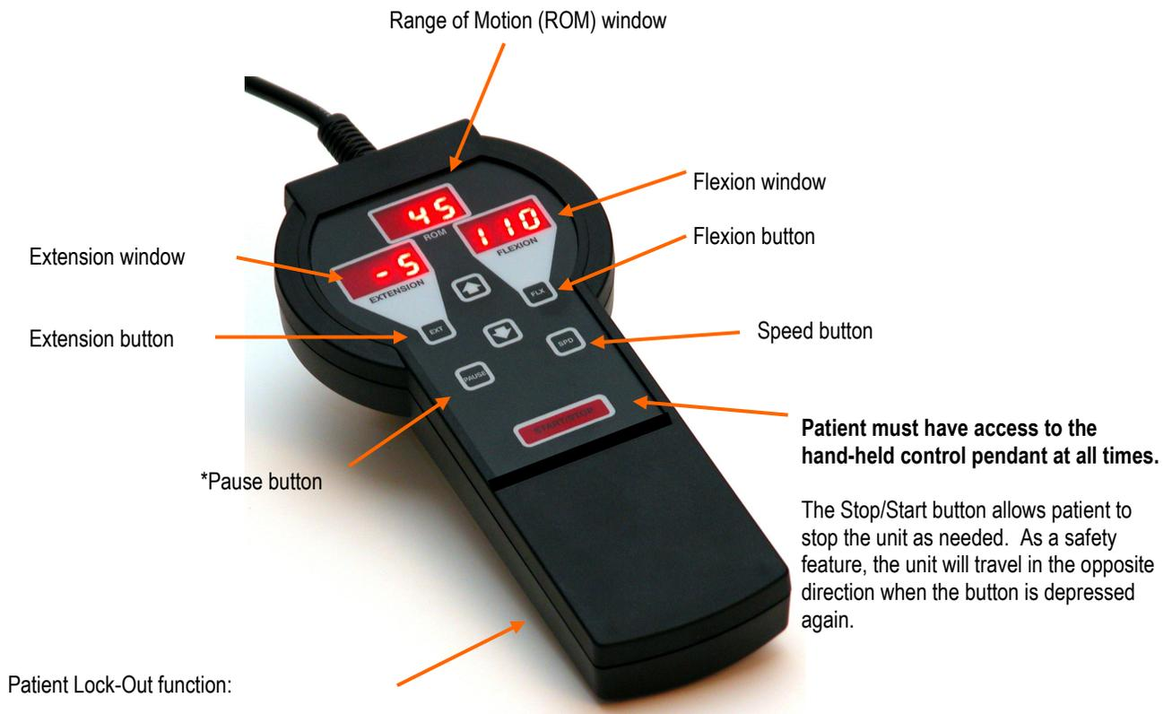
The Stop/Start button allows patient to stop the unit as needed. As a safety feature, the unit will travel in the opposite direction when the button is depressed again.
